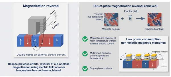
$Direct observation of magnetization \ reversal \ by \ electric \ field \ at \ room \ temperature \ in \ Co-substituted \ Bismuth \ ferrite \ thin \ film \ and \ reversal \ film \ fil$
