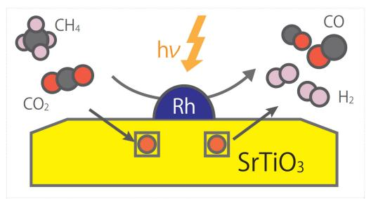
Figure 1 Photocatalytic uphill conversion of natural gas beyond thermal reaction systems
