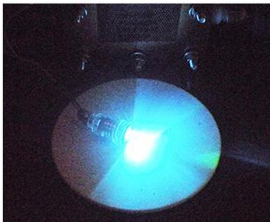
Figure 6. Electric power generated by a fuel cell with H<sub>2</sub>ase S-77.
