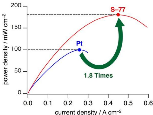
Figure 4. Power density *versus* current density produced from fuel cells with platinum and H<sub>2</sub>ase S-77 as the anode catalyst and platinum as the cathode catalyst.
