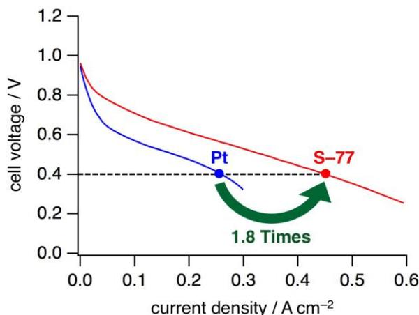
Figure 3. Cell voltage *versus* current density produced from fuel cells with platinum and  $\text{H}_2\text{ase S-77}$  as the anode catalyst and platinum as the cathode catalyst.
