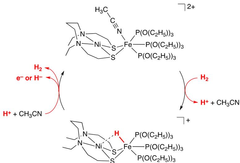
Figure 4. Electron extraction from hydrogen gas with the nickel-iron catalyst (this work)
