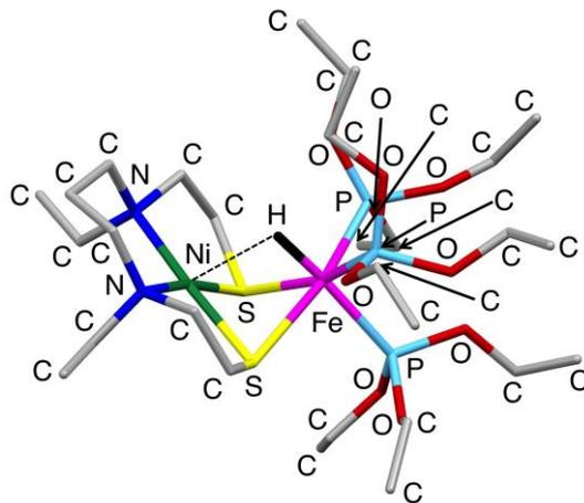
Figure 3. X-ray structure of the nickel-iron catalyst (this work)
