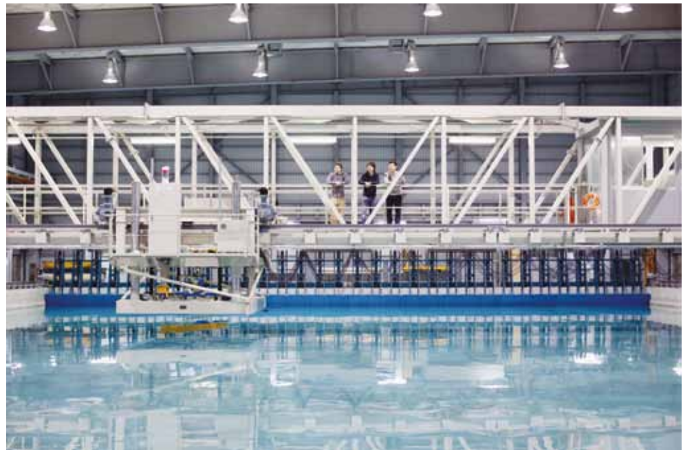
Computerized planar motion carriage (CPMC) and plunger type wave maker installed in the Seakeeping and Maneuvering Basin. These facilities are used for model experiments to study ships and floating bodies.
