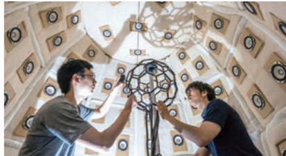
"Sound Cask," a three-dimensional sound field reproduction and recording system
