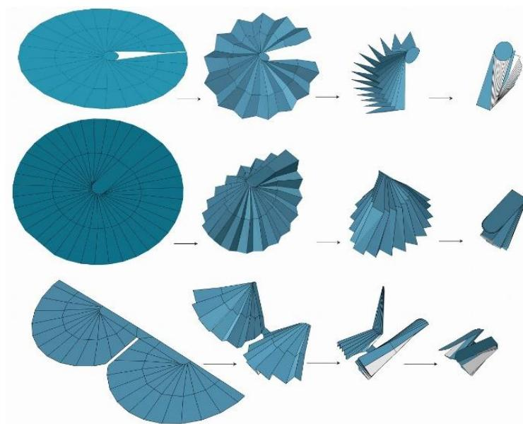
**Examples of customised earwig-inspired fans made using the new design software. Above: two models of earwig fans for use in deployable structures such as antenna reflectors or umbrellas. Below: deployable wings for a micro air vehicle. Note the high compactness of the fans when fully folded. Credit: Kazuya Saito.**
