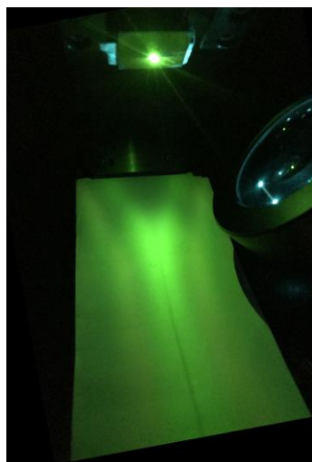
A layer of perovskite is shown lasing under continuous operation at room temperature.
