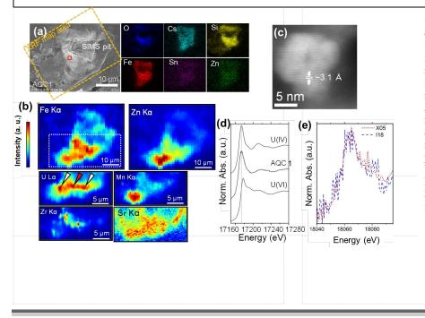
(a)SEM image with EDX elemental maps of a CsMP. (b) Synchrotron micro-focus X-ray fluorescence (µXRF) elemental maps. (c) HR-HAADF-STEM image of a discrete U dioxides nanoparticle. (d) Uranium *L*<sub>3</sub>-edge X-ray absorption near-edge structure (XANES) of a discrete point, indicated by the red arrow in (b). The spectrum is plotted alongside U(IV) and U(VI) oxide standards. (e) Discrete-area Pu L3-edge XANES collected from the point indicated by the red arrow.
