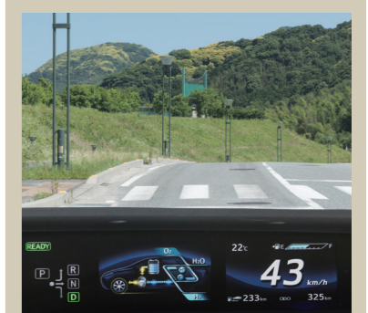
MIRAI's LCD panel showing the energy balance while running
