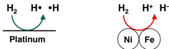
Figure 5. Homolytic and heterolytic activation of hydrogen molecule by platinum and H<sub>2</sub>ase S-77.
