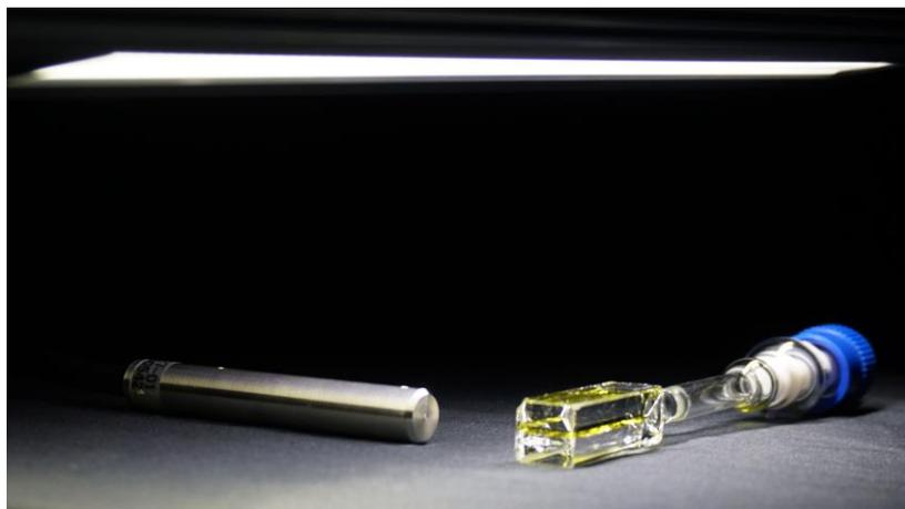
The molecular system in the glass tube on the right efficiently upconverts visible light even from typical LEDs into ultraviolet light through triplet-triplet annihilation.
