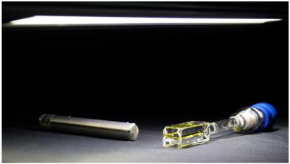
The molecular system in the glass tube on the right efficiently upconverts visible light even from typical LEDs into ultraviolet light through triplet-triplet annihilation.
