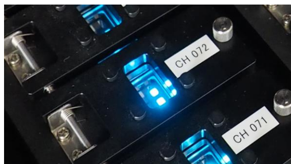
Highly efficient, pure-blue organic light-emitting diodes are tested to measure their lifetime.
