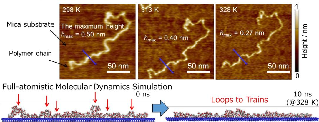
Atomic force microscopy height images for a single polymer chain on mica and snapshots of a polymer chain obtained by a molecular dynamics simulation upon heating.
