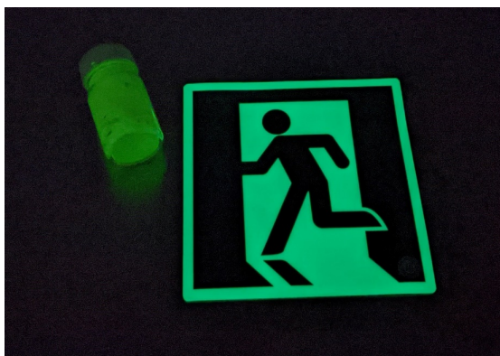
Glow-in-the-dark materials and a common application in exit signs.
