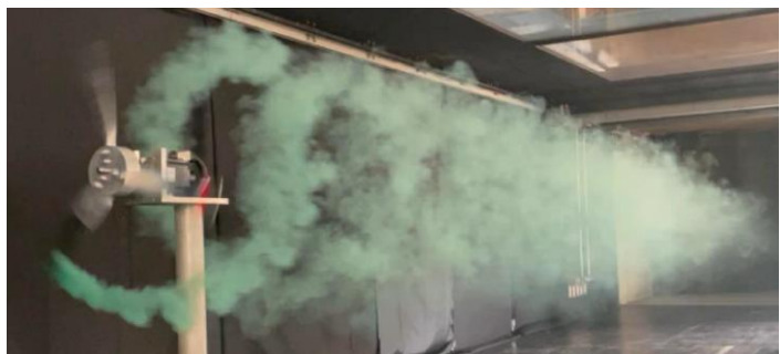
Visualization example of wind turbine wake phenomena using large wind tunnel facilities
