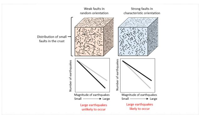
Fig. 2. When the earth's crust contains many weak faults in random orientations, large earthquakes are unlikely to occur. However, when the earth's crust contains many strong faults that are oriented in characteristic direction, there is a higher likelihood that a large earthquake could occur.
