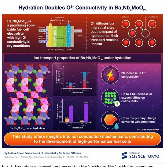
Fig. 1. Hydration-enhanced ion transport in Ba<sub>7</sub>Nb<sub>4</sub>MoO<sub>20</sub>. Ba<sub>7</sub>Nb<sub>4</sub>MoO<sub>20</sub>, a ceramic electrolyte with potential for low-temperature fuel cells, becomes nearly twice as conductive when exposed to water vapor at 500 °C. The improvement is driven by enhanced oxide-ion mobility in the material and could lead to more efficient and durable fuel cells. (Institute of Science Tokyo)
