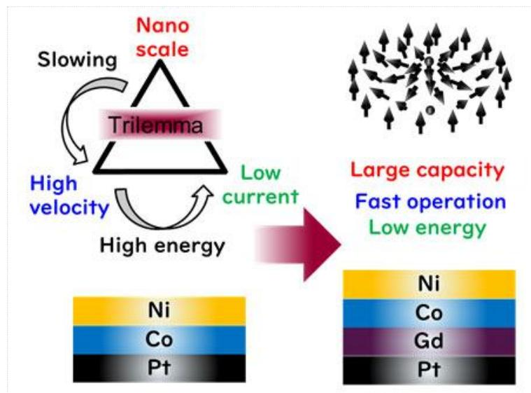
**Fig. 1. Toward energy-efficient information technology with magnetic skyrmions**
