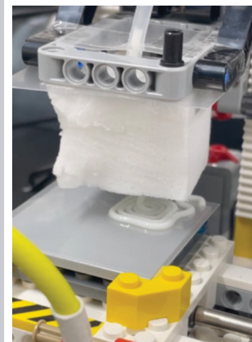
▲ The bioprinter in action. The bioink is passed through the microwave emitter, which heats it with varying microwave frequencies. The resulting gel is then printed onto the platform. (Kyushu University/Shuntaro Tsubaki)
