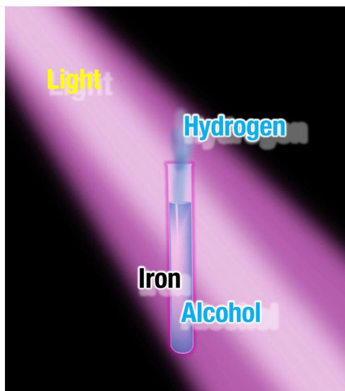
Fig. 1. Conceptual illustration of light-driven hydrogen generation. An illustration of the reported new method of generating hydrogen gas using alcohol, iron ions, and UV light. (Kyushu University/Matsumoto Lab)
