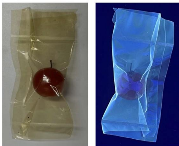
FIG.2 Biodegradable film with carbon quantum dots fluoresces under UV light
