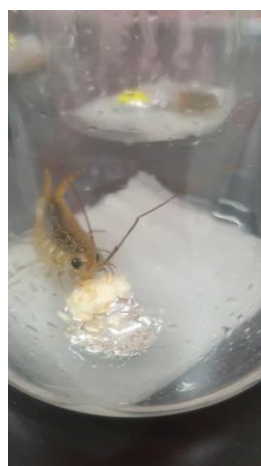
Fig. 2. Wharf roach consuming EPS. A wharf roach consuming EPS during the team’s experiments
